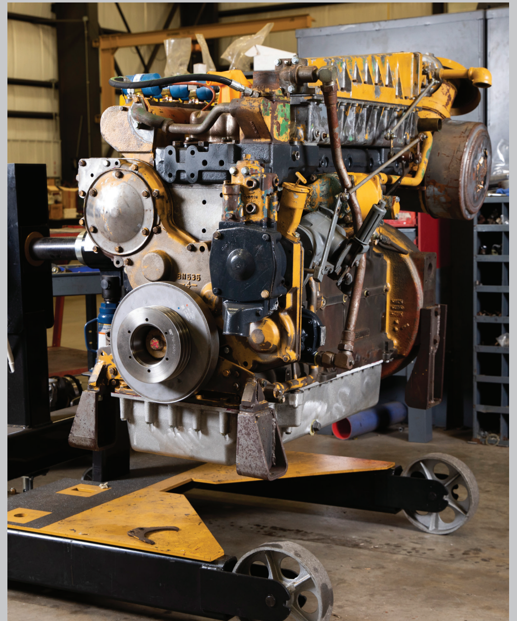
3306TA engine in Houston Reman Center
